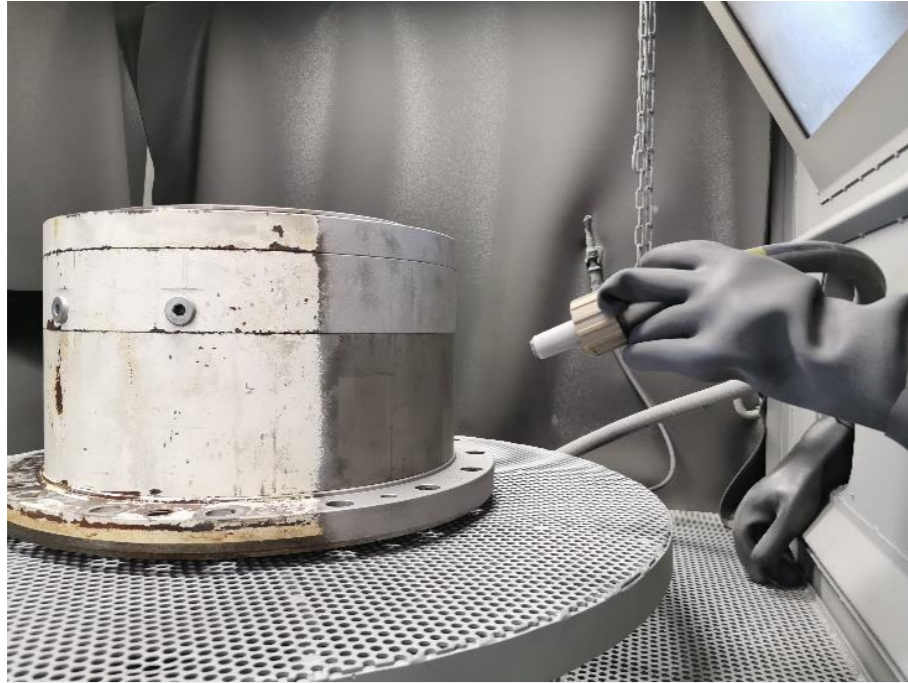
Conservative sand blasting for removal of painting
