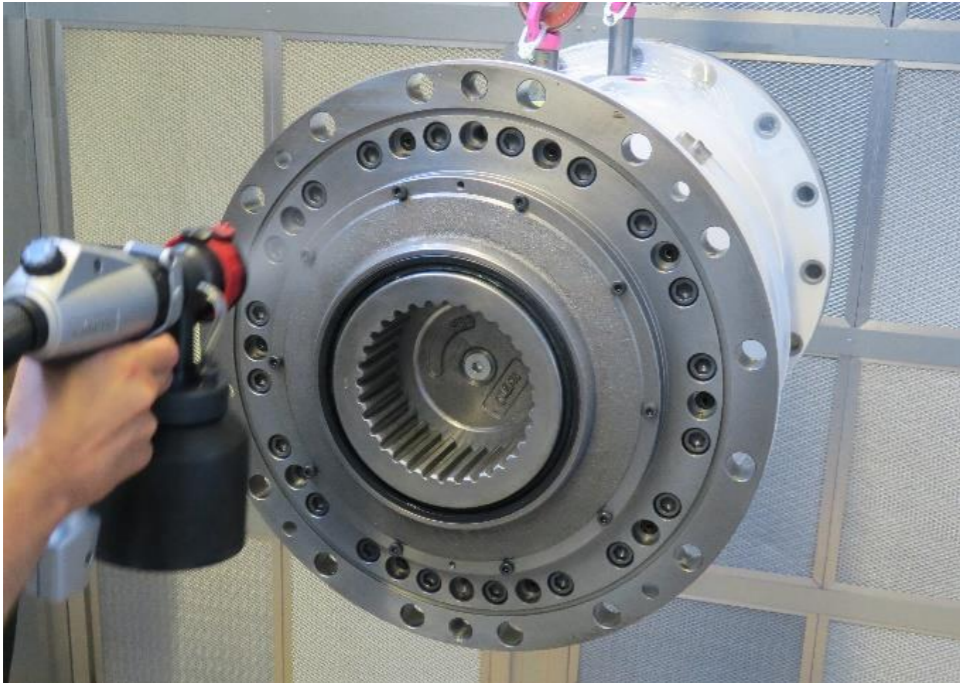
Application of corrosion protection for the transport
